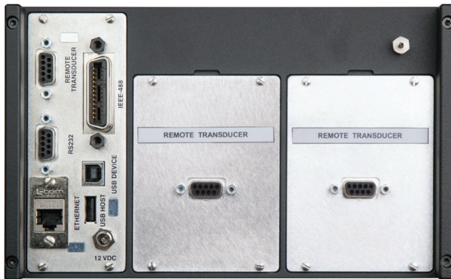
Figure 5.4 B - Two remote transducer interface connections installed
