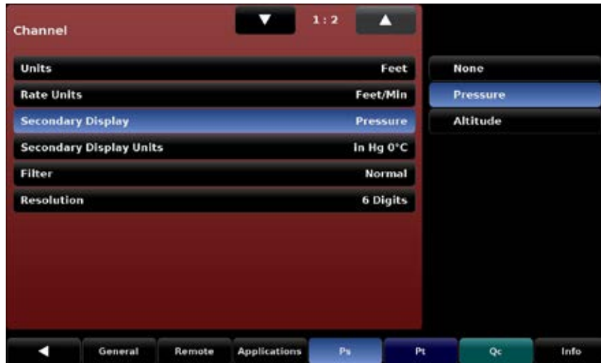
Figure 7.3.3 - Ps Secondary Display set to [Pressure]
