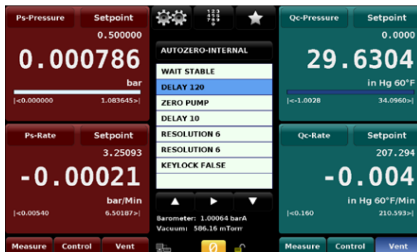
Figure 6.2.15c - Zero Sequence, 120 second delay
