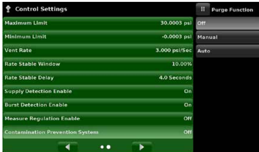
Figure 8.9.2.3-B - Contamination Prevention System
