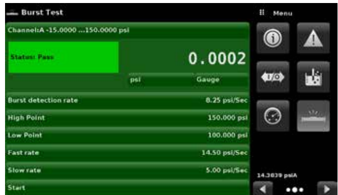
Figure 6.4.14-C - Burst Test Complete (No Burst)
