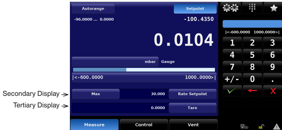
Figure 6.2.9a - Secondary and Tertiary Displays
