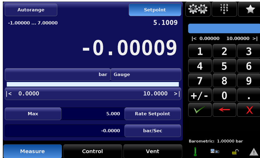
Figure 6.2.4 - Output Pressure Setpoint
