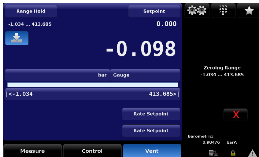
Figure 6.2.14-A Zero Button in Gauge
