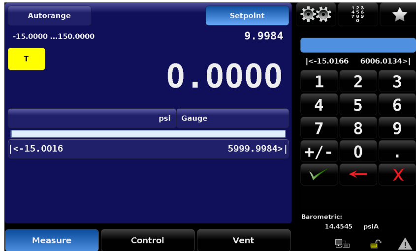
Figure 6.2.14-C Tare Button active
