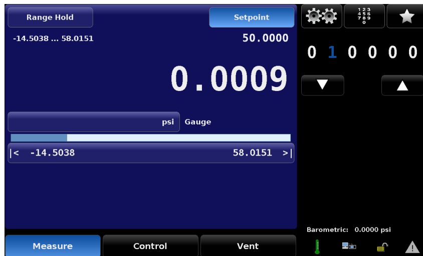
Figure 6.2.6.4 - Digital Step Screen
