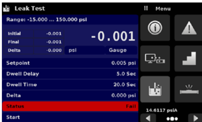
Figure 6.4.11-A – Leak test fail (left) & Leak test pass (right)
